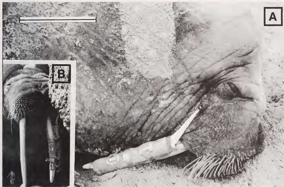
Fig. 2. The T-2028 satellite transmitter used in 1990 (A); close up view (B); scale = 25 cm. The transmitter which weighed 0.305 kg was glued into a stainless steel cylinder with polyurethane and two-component epoxy glue, resulting in a total weight of the unit of 0.750 kg
